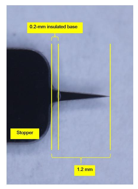
Figure 3 / S type needle used for the procedure. The length is 1.2mm and the shoulder of the base part acts as a stopper to prevent the needle from getting too deep into the skin. Since 0.2mm from the base part is treated with insulation coating, the epidermis is protected.
